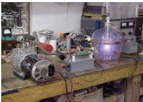
Inexpensive Benchtop Inertial Electrostatic Confinement Demonstration & Test Cell
