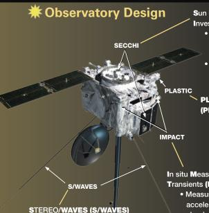
Sun Earth Connection Coronal and Heliospheric Investigation (SECCHI)
