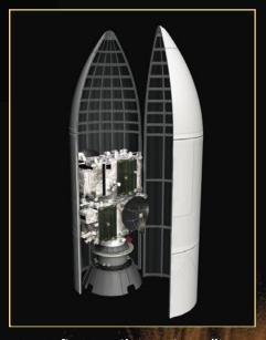
A spacecraft separation system allows one STEREO observatory to sit atop the other within the third stage of the Delta II launch vehicle.
