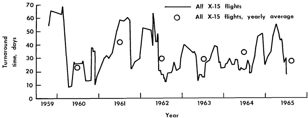
Figure 2.— Average turnaround time per aircraft (based upon average of five successive flight groups).
