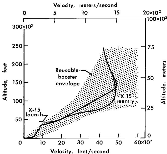
Figure 1.— Comparison of a typical X-15 profile with reusable-booster envelope.
