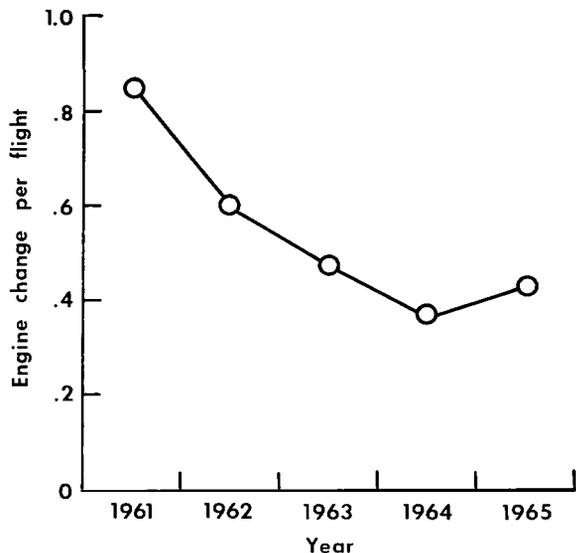
Figure 4.— Engine changes per flight, by years.
