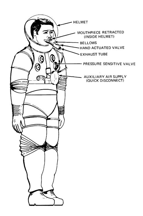
FIGURE 1 - VOMIT REMOVAL APPARATUS FOR EVA PRESSURE SUIT.
