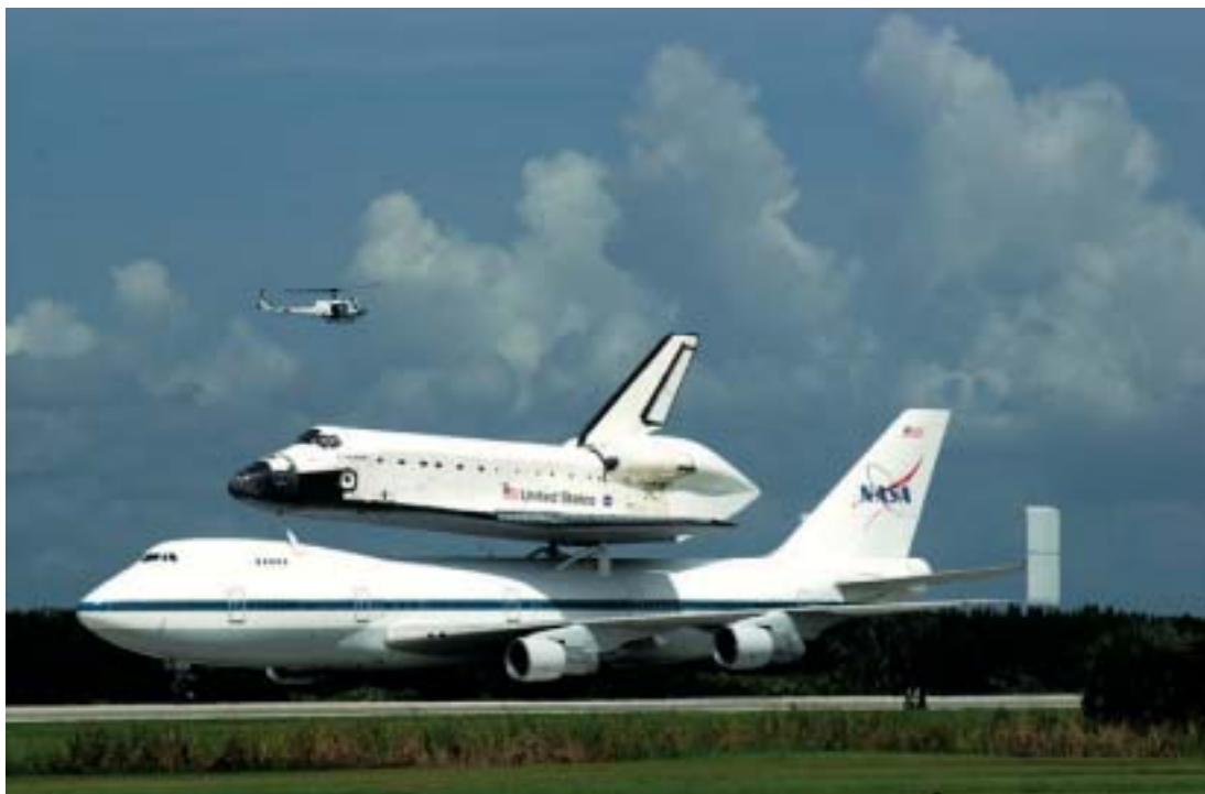
Space Shuttle Endeavour lands on runway 15 at KSC's Shuttle Landing Facility atop a modified Boeing 747 Shuttle Carrier Aircraft. The cross-country ferry flight became necessary when three days of unfavorable weather conditions at KSC forced Endeavour to land at Dryden Flight Research Center, Edwards Air Force Base, Calif., on June 19 following mission STS-111.
