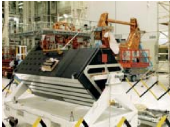
The Advanced Camera for Surveys (ACS) launched on STS-109 for maintenance of the Hubble Space Telescope. (See page 1.)
