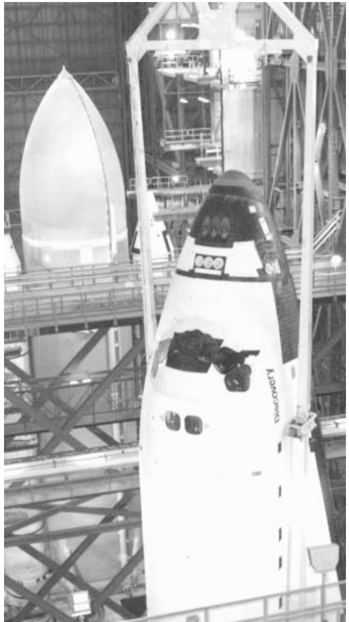
An orbiter is raised to a vertical position and lifted for mating to the external tank and solid rocket boosters in the Vehicle Assembly Building.
