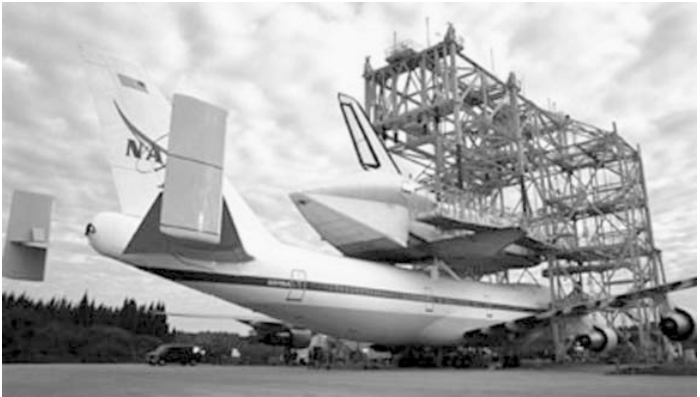
The mate/demate device at the Shuttle Landing Facility lifts an orbiter from the Shuttle Carrier Aircraft used in ferry operations. Movable platforms provide access to orbiter components.
