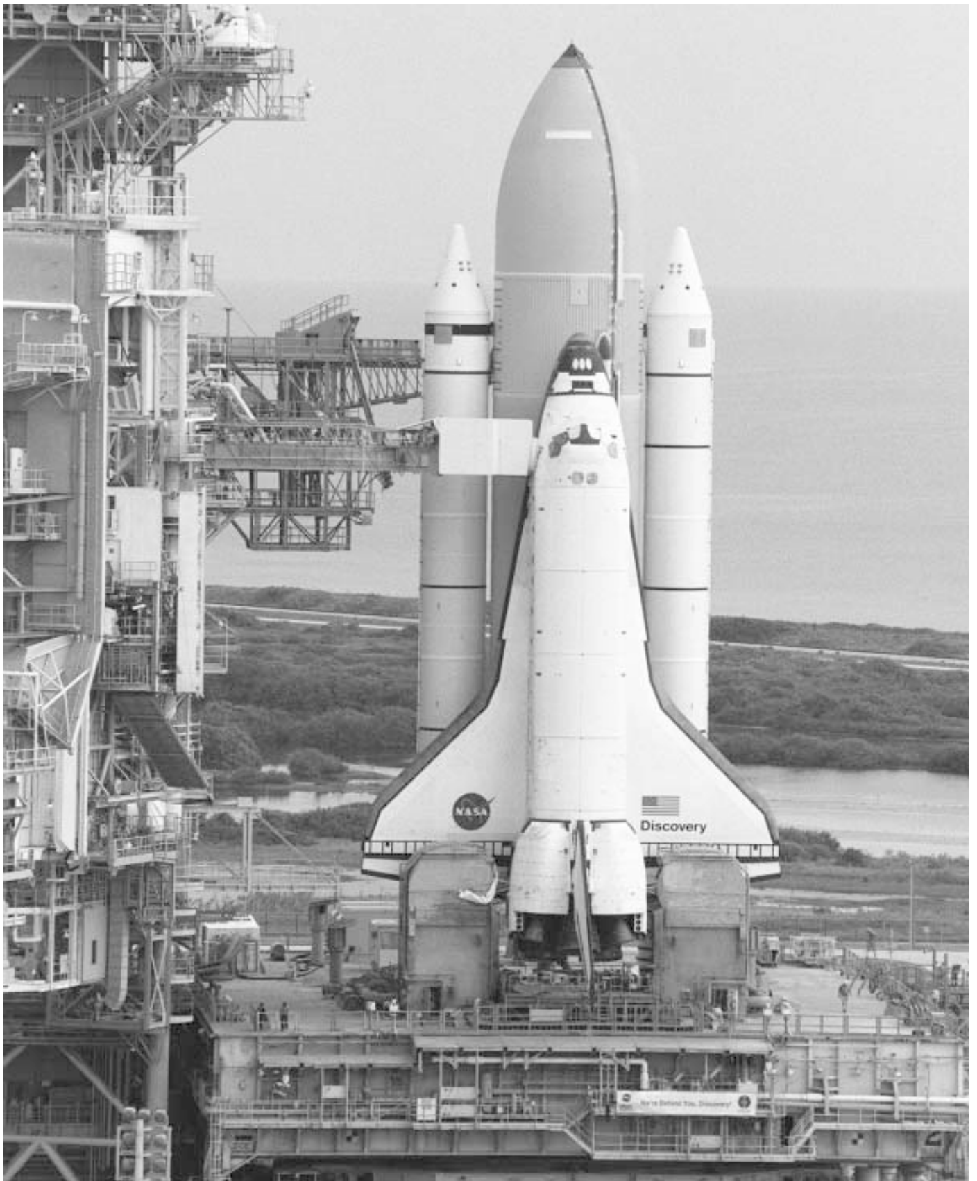
Each side of the orbiter at the launch pad is connected to a Tail Service Mast, either side of the engine nozzles. The Mast provides propellant-loading umbilicals and establishes connections to ground support equipment.
