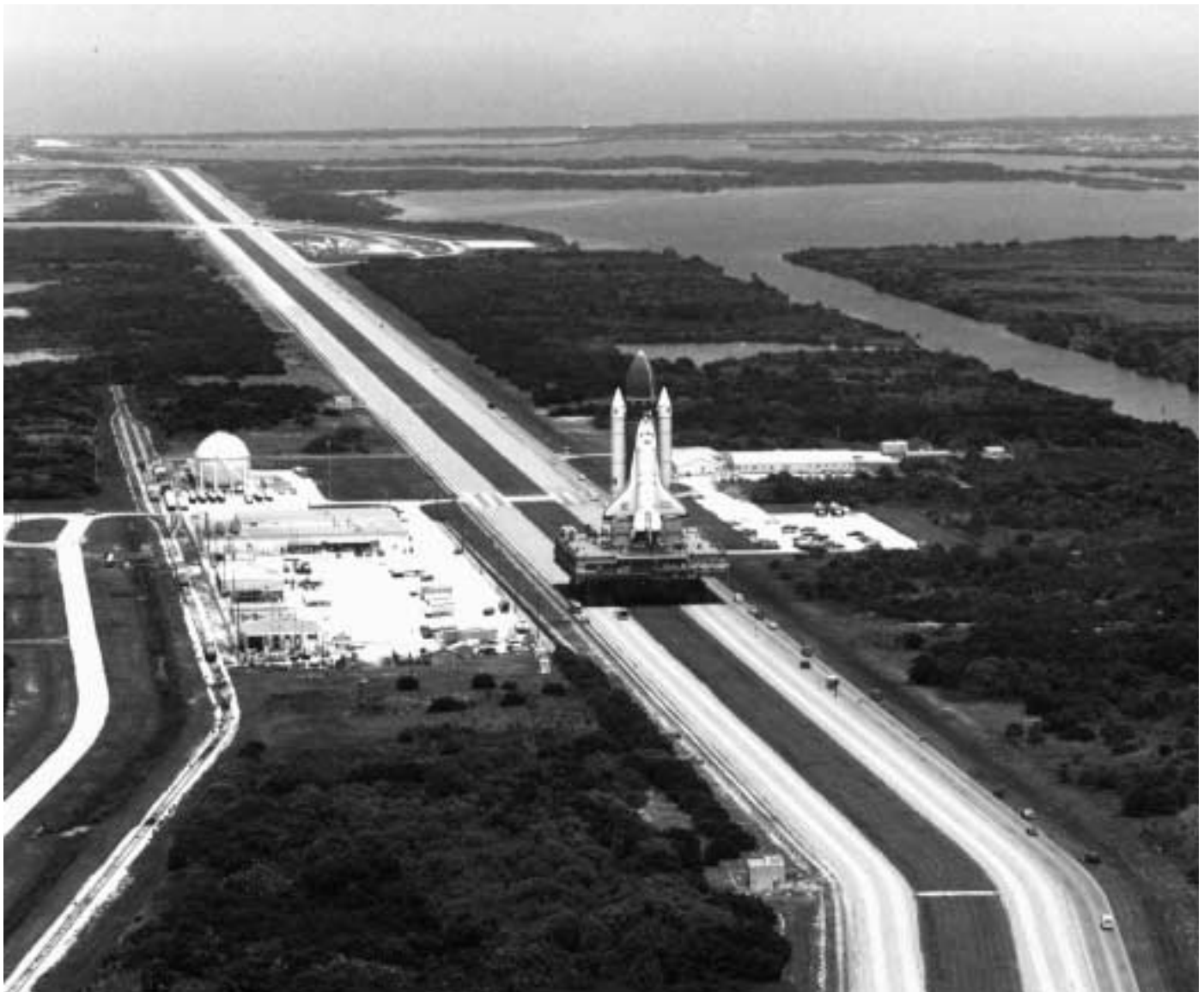
The Space Shuttle assembled on the Mobile Launcher Platform moves slowly on the Crawlerway between the Vehicle Assembly Building and the launch pads.
