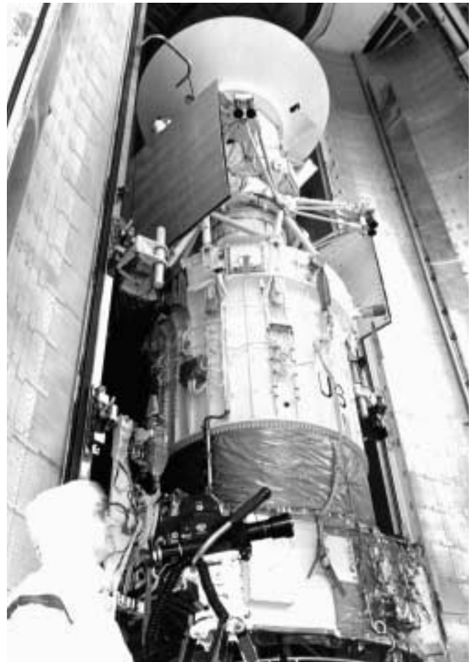
Spacecraft are loaded into the Payload Changeout Room at the launch pad after delivery in the Payload Canister. Here, the spacecraft Magellan is prepared for installation at the pad before beginning its journey to Venus.
