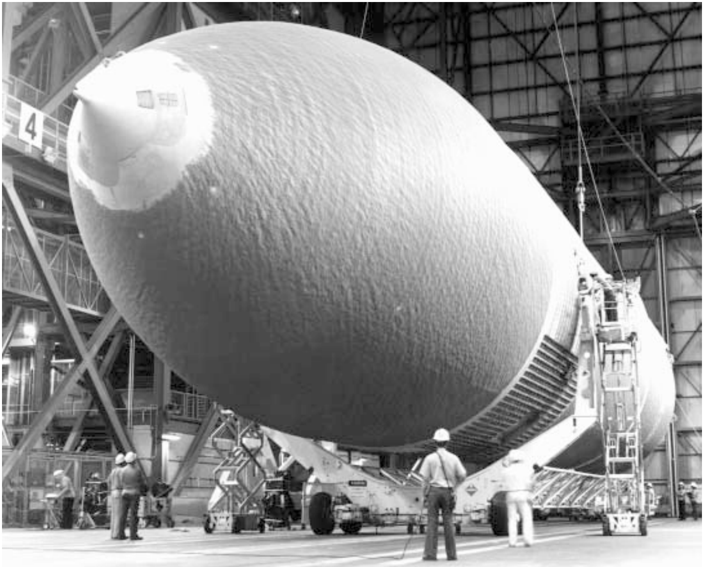
The external tank rests on its trailer in the transfer aisle of the Vehicle Assembly Building after arriving by barge at Kennedy Space Center.
