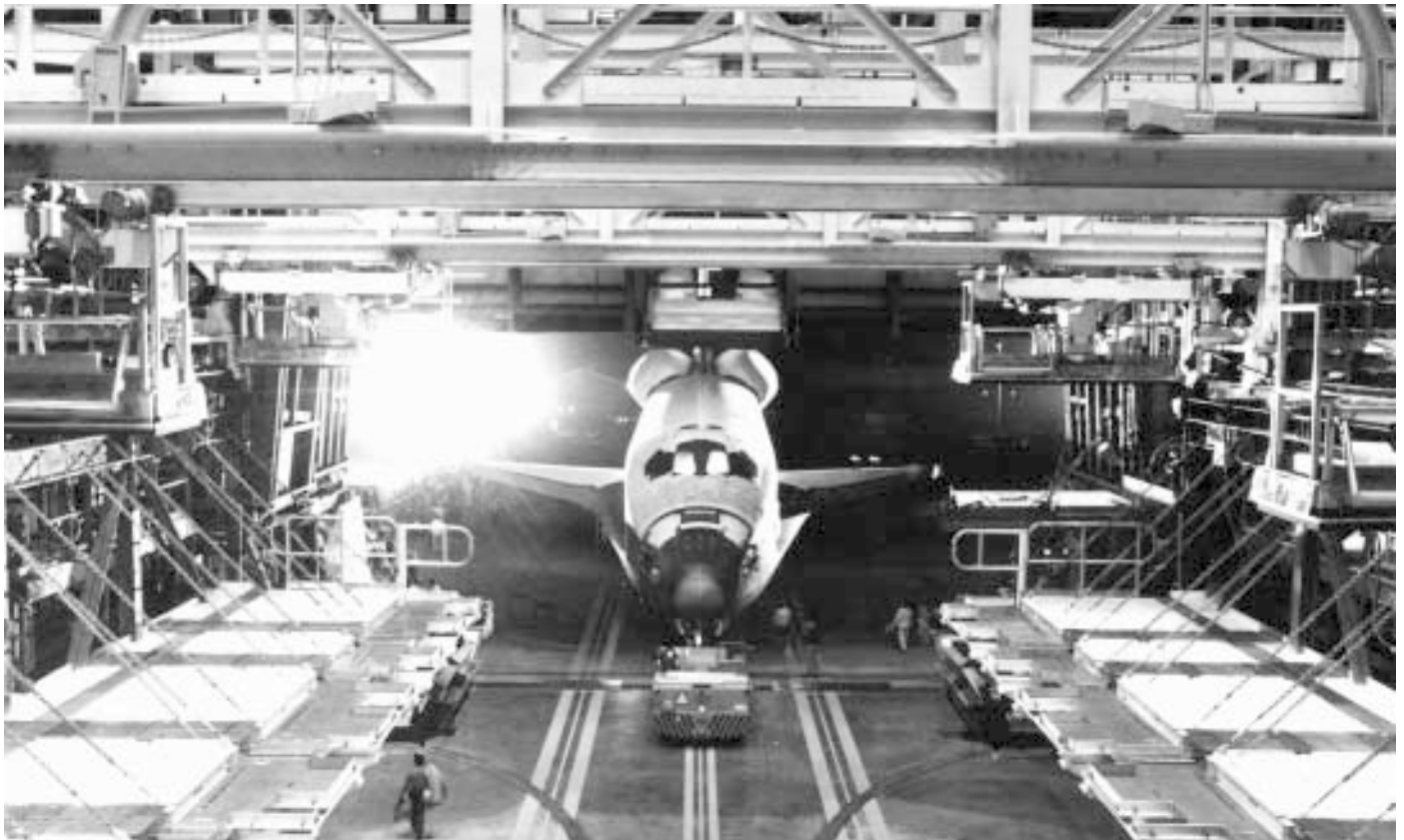
Processing for a mission begins when an orbiter is towed into one of these Orbiter Processing Facility bays at KSC.
