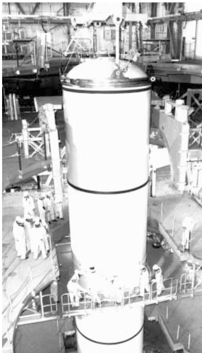
Assembly of the Space Shuttle flight components such as this solid rocket booster takes place in high bays 1 or 3 of the Vehicle Assembly Building. The two boosters are stacked on the Mobile Launcher Platform. The external tank is then mated to the boosters, and the orbiter is the final component added.
