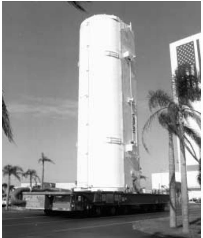
The Payload Canister Transporter can transport payloads in the Canister either vertically or horizontally.
