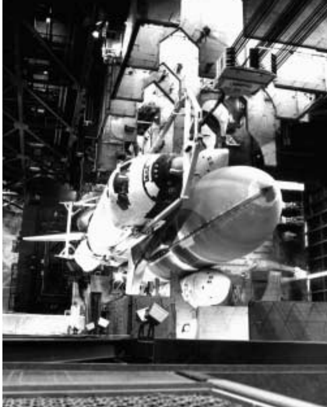
A huge crane lowers the orbiter into position to be attached to the external tank in the Vehicle Assembly Building.
