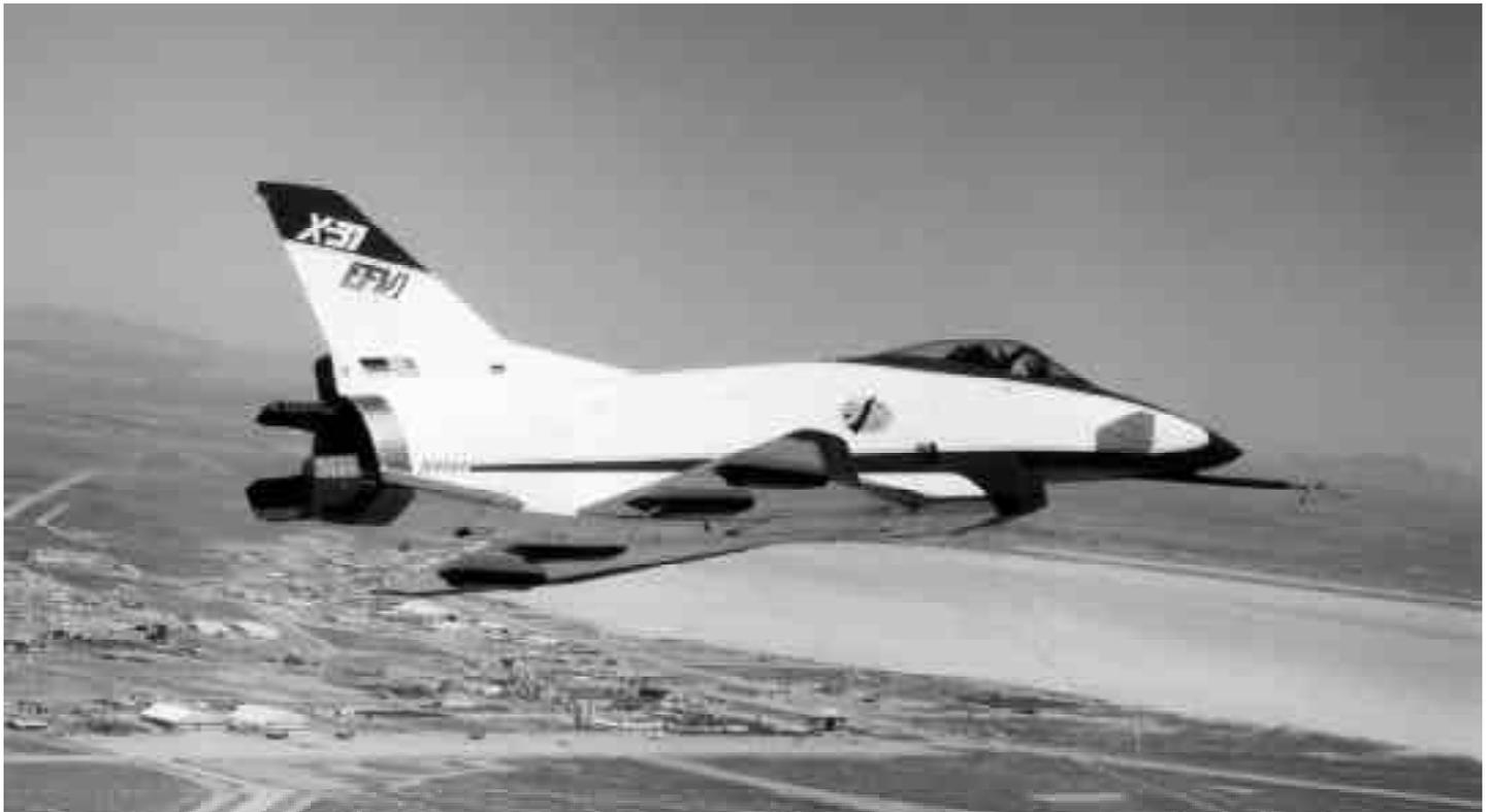
X-31 #1 flying over Edwards. Notice the three thrust-vectoring paddles at the rear of the aircraft. (NASA photo EC 93-42152-8)
