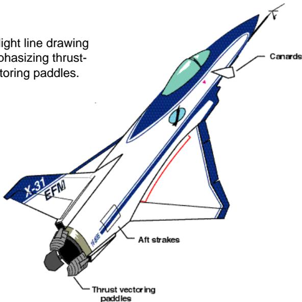
The X-31 operated with a digital fly-by-wire flight control system. It included four digital flight control computers with no analog or mechanical back-up. Three synchronous main computers drove the flight control surfaces. The fourth computer served as a tie-breaker in case the three main computers produced conflicting commands.
