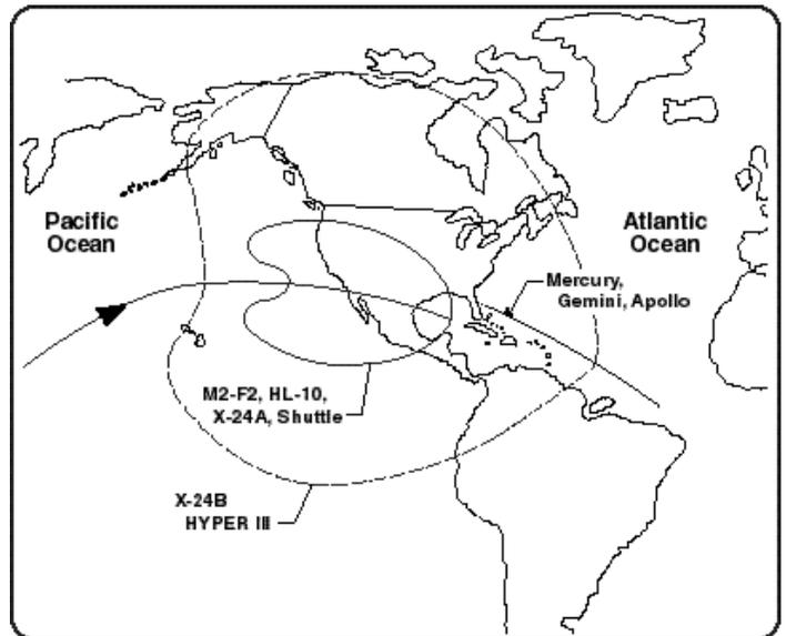
*Orbital entry footprints (lateral and longitudinal maneuverability) of lifting bodies and spacecraft. (Note the very small area for the Mercury, Gemini, and Apollo capsules as compared with the lifting bodies and the Space Shuttle.)*
