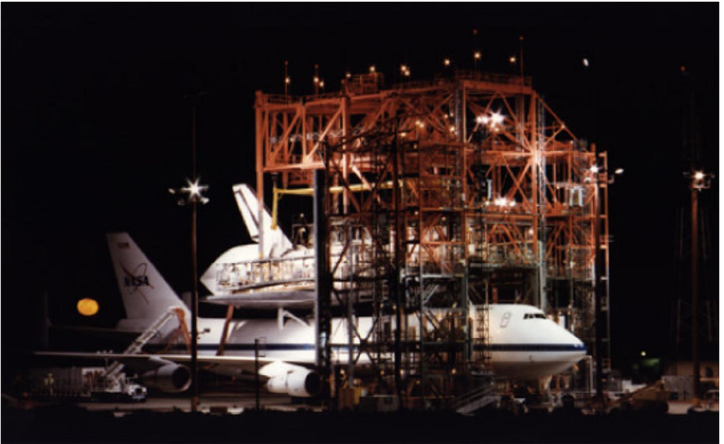
*EC96 43493-1 The Space Shuttle Atlantis receives post-flight servicing in the MDD following its landing at the NASA Dryden Flight Research Center, Edwards, Calif., March 31, 1996. Atlantis is shown atop Shuttle Carrier Aircraft 905.*
