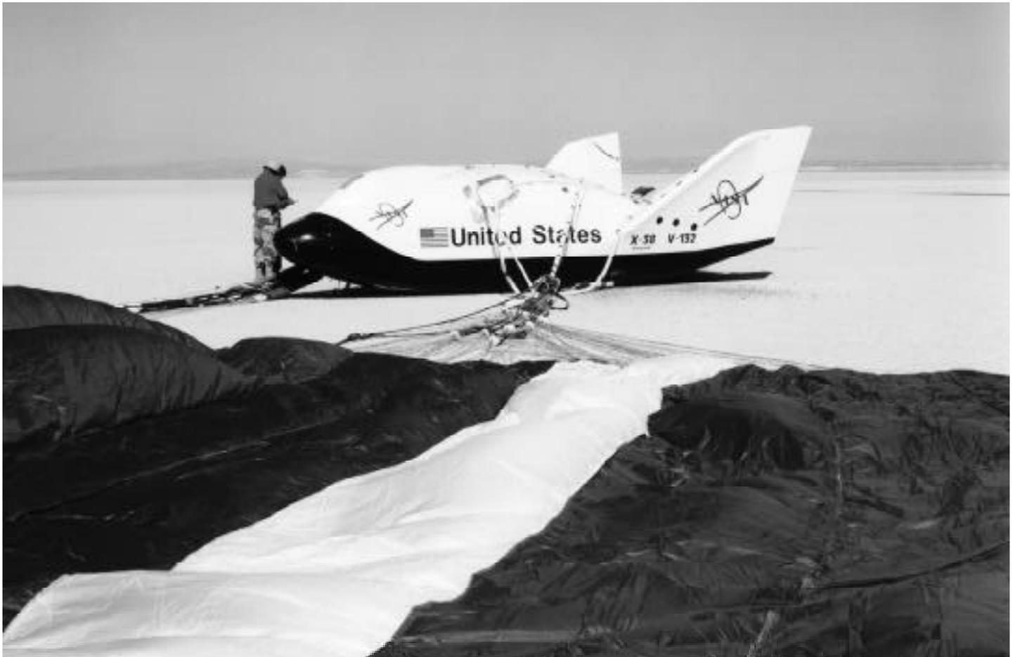
The X-38 project is a series of five prototype research vehicles developing technology to build and operate a space station crew return vehicle (CRV). The wingless CRV, when operational, would be the first reusable human spacecraft to be built in more than two decades.
