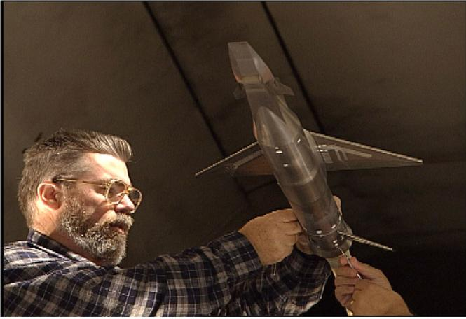
**During the X-43A investigation, researchers conducted many tests including wind tunnel tests of the full-stack model.**
