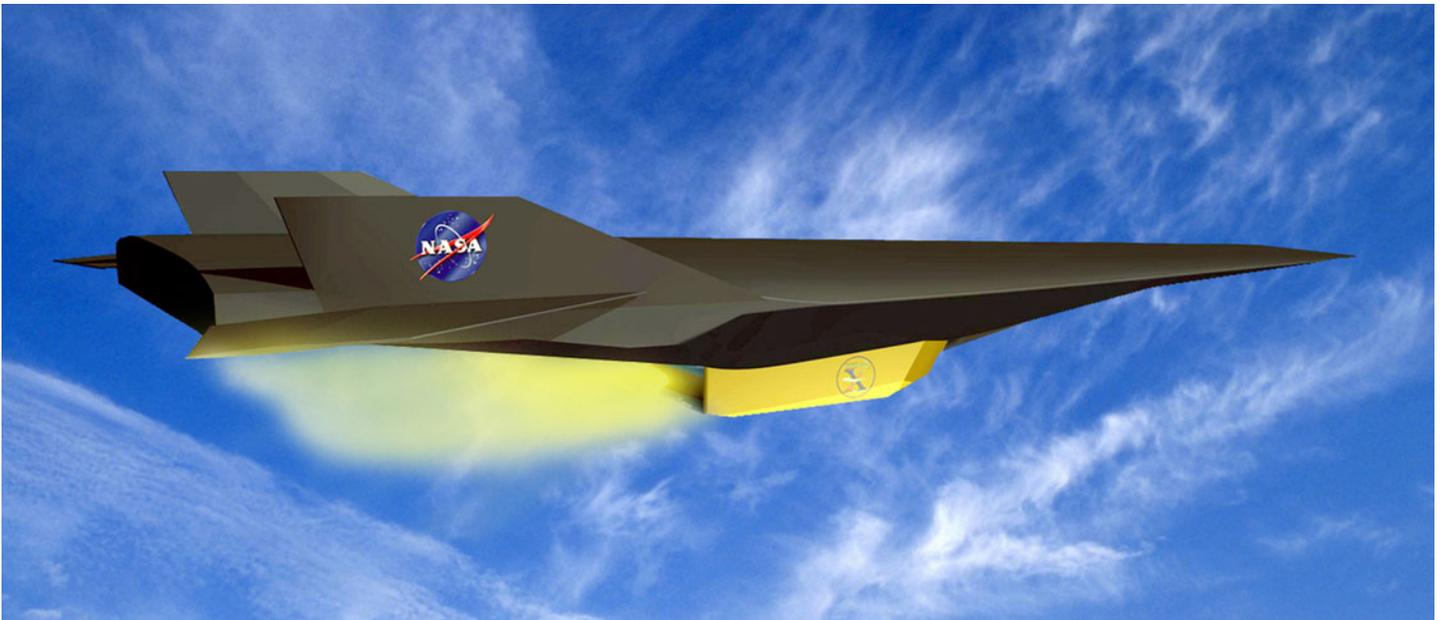
The Hyper-X program aims to significantly expand the boundaries of air-breathing flight by being the first to fly a "scramjet" powered aircraft at hypersonic speeds.
