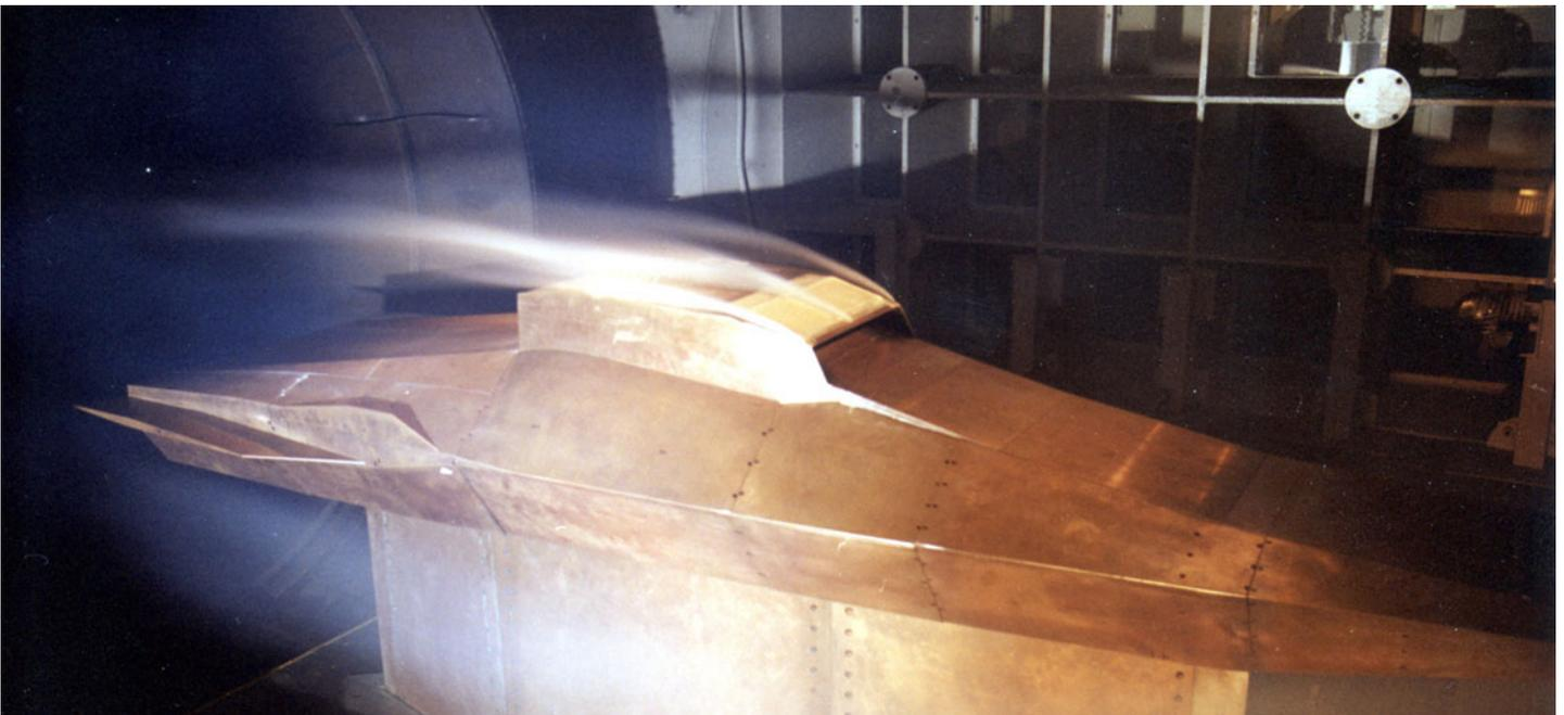
**Wind tunnel tests show good aerodynamic and propulsion performance for the Hyper-X configuration. Shown here is a Mach 7 test of the full-scale model with spare flight engine in Langley's 8-Foot High Temperature Tunnel.**
