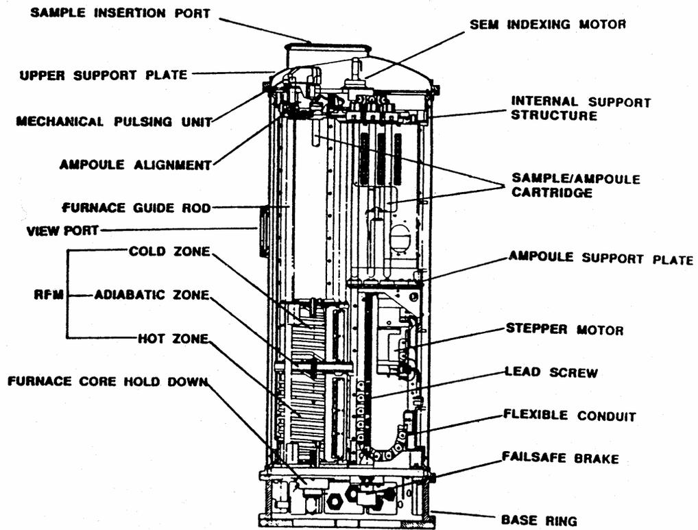
CGF INTEGRATED FURNACE EXPERIMENT ASSEMBLY (IFEA)
