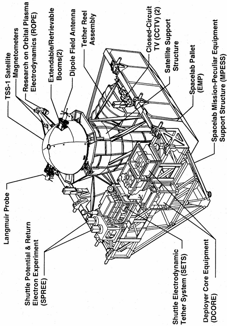
The primary objectives of the first tethered satellite mission are to evaluate the capability to safely deploy, control and retrieve a tethered satellite, to validate predictions of the dynamic forces at work in a tethered satellite system and to conduct exploratory electrodynamic science investigations and demonstrate the capability of the system to serve as a facility for research in geophysical and space physics.
