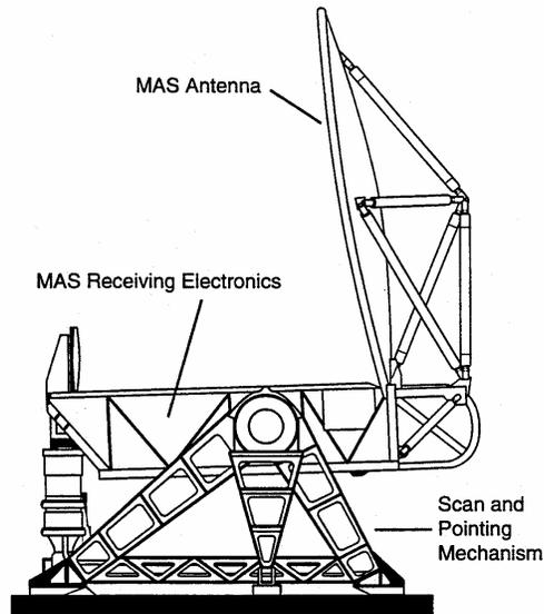
**Millimeter-Wave Atmospheric Sounder (MAS)**
