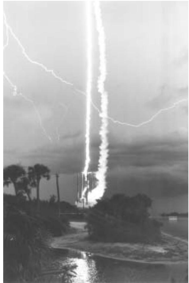
The lightning event begins when lightning strikes the 3,000-foot copper wire being trailed from the 3-foot-tall rocket. The wire is then vaporized as it follows the path to a lightning rod attached to the launcher. As the wire burn dissipates, it creates an effect called irosary bead lightning. This can be the prelude to natural lightning restrikes. The initiation of a wire burn can also induce natural intercloud lightning during the event, as seen in this sequence.
