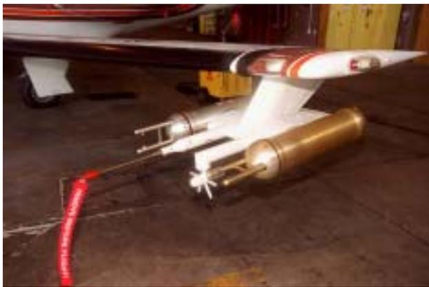
Attached to the wing of a Cessna Citation aircraft are cloud physics probes that measure the size, shape and number of ice and water particles in clouds. The plane is also equipped with field mills, used to measure electric fields. The plane is being flown into anvil clouds in the KSC area as part of a study to review and possibly modify lightning launch-commit criteria.
