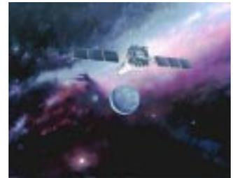
With its combination of four pairs of ultra smooth, high-resolution mirrors and efficient X-ray detectors, Chandra makes images at least thirty times sharper than any previous X-ray telescope. The High Resolution Camera, and the Advanced CCD Imaging Spectrometer record images electronically, and two transmission gratings enable scientists to make precise measurements of the energies of incoming X rays.
