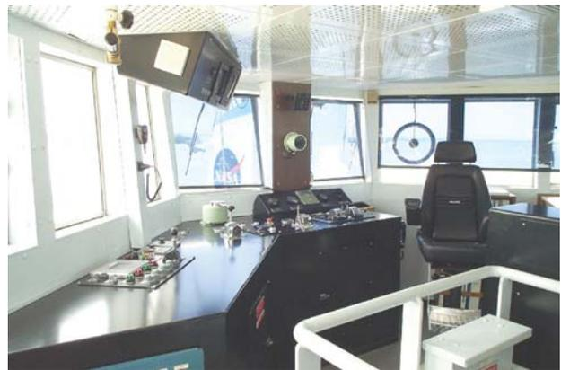
The forward area of the bridge (left) is for operation of the ship itself. Such state-of-the-art equipment as the Global Positioning System for precise navigation is located here. Booster retrieval operations are controlled from the aft bridge of the ship (right). Equipment located here includes hookups for communicating with the divers, forward deck and the other retrieval ship, along with a wind gauge, stern/bow thruster controls and radar.
