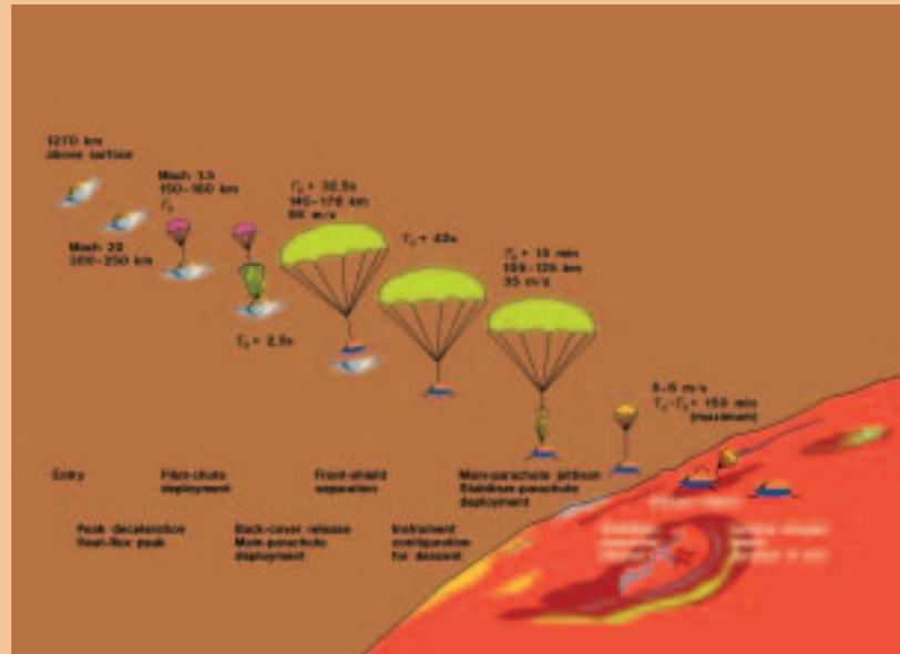
The shell of the descent module falls away and exposes the scientific instruments to Titan's atmosphere at a height of about 160 km. The atmospheric temperature may then be about -120°C.
