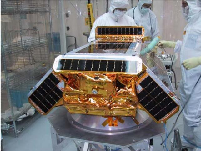
CHIPS' six apertures for observing the Interstellar Medium are located just below the small disk in the center of the forward end. The black rectangles are solar cells. (Photo UCB)
