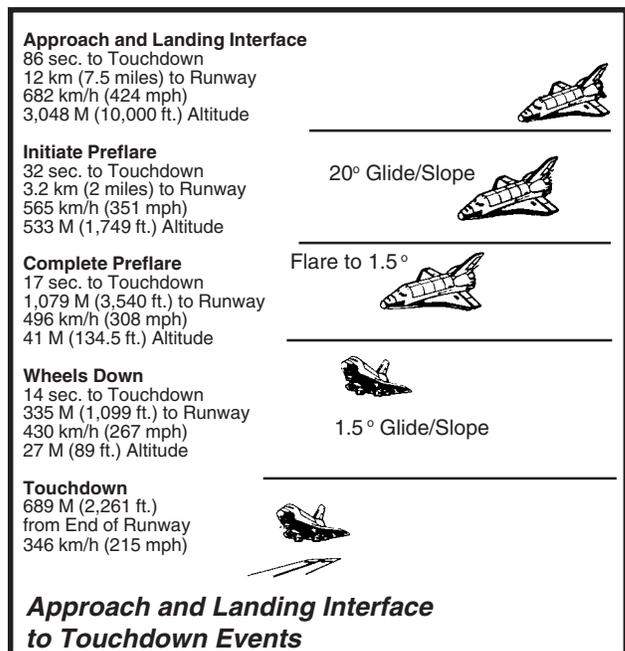
These two charts represent an example of the sequence of events or flight milestones from the deorbit maneuver of the orbiter through touchdown. The times, distances and speeds will vary for different missions, according to a variety of factors such as mission inclination, trajectory and glide slope.
