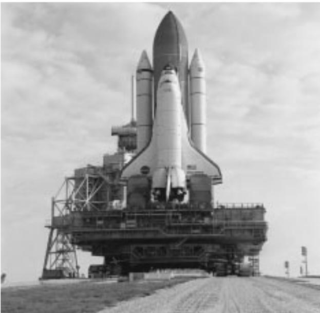
below). The MLP is parked on pedestals permanently located at the pad and is the platform from which the Shuttle is launched. Several MLP systems interface with pad systems. These include the Sound Suppression System and the propellant transfer lines for the external tank. Helium and nitrogen, as well as ground electrical power and connections for vehicle data and communications, also are established through the tail service masts of the MLP.
