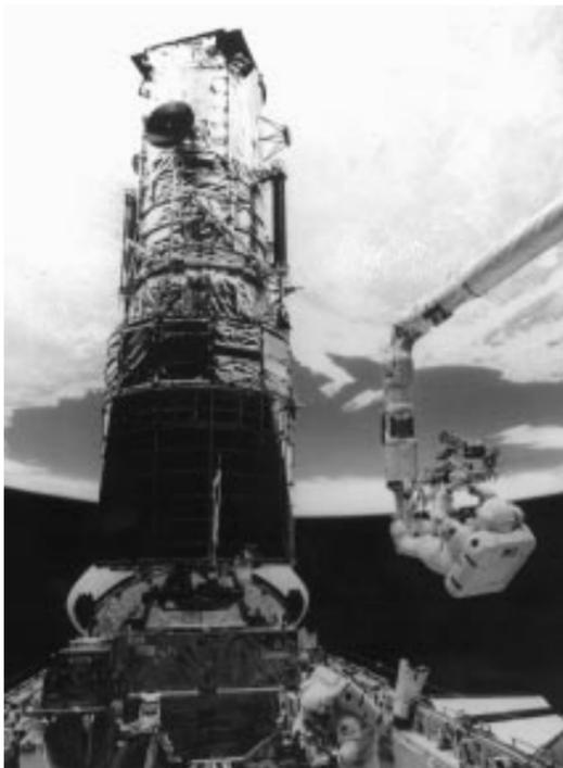
The Shuttle's usefulness as a platform for on-orbit servicing of spacecraft was demonstrated during the STS-61 Hubble servicing mission in 1993. Spacewalking astronauts successfully completed repairs and upgrades to the Hubble telescope while it was temporarily stored in the orbiter Endeavour's payload bay.
