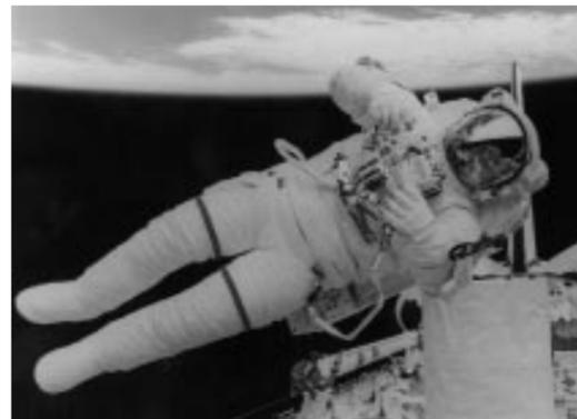
During the first untethered space walk in 10 years, Mission Specialist Mark Lee tests the new Simplified Aid for Extravehicular Rescue (SAFER) system. The 28th space walk of the Shuttle program took place on Mission STS-64 in September 1994.
