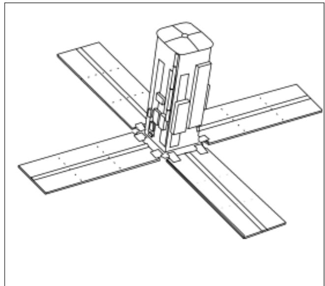
*Spartan Lite with its solar arrays deployed*
